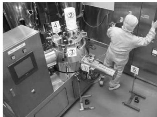
Fig.14 Measuring leaked powder
